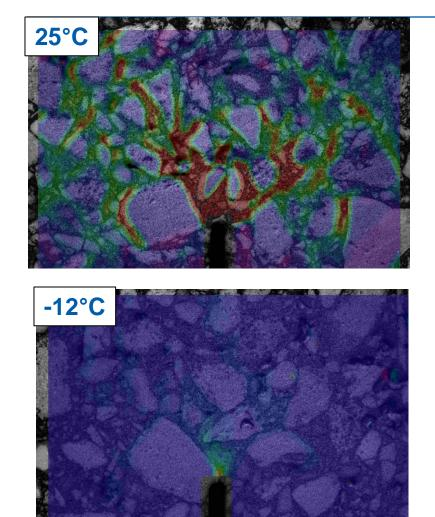
Diffused damage at intermediate temperature
