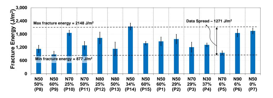
SCB fracture energy results for the same mixes at 25°C using displacement control at 50 mm/min
